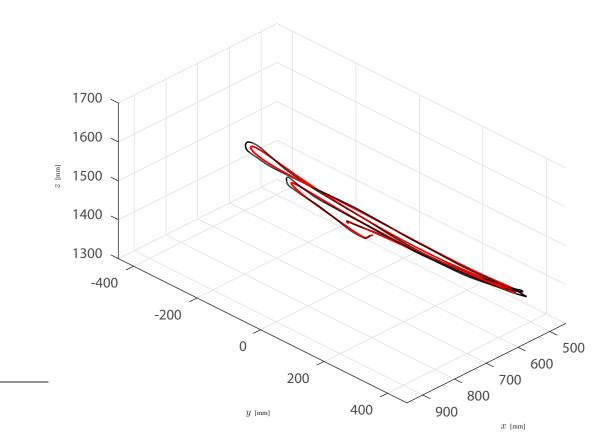
Fig. 10. Geometric path of a linear movement of the user tracked by the motion capture system. The black line is the original trajectory while the red line represents the trajectory filtered by the harmonic smoother.
