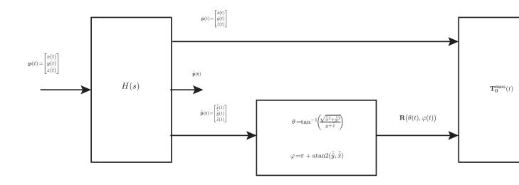
Fig. 8. Feed-forward controller for sloshing compensation based on the harmonic smoother.
