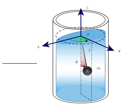
Fig. 7. Spherical pendulum modelling the sloshing dynamics in a liquid-filled vessel that moves along a 3D trajectory.
