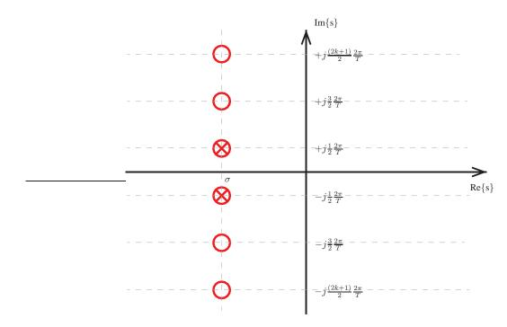
Fig. 4. Pole-zero map of the damped harmonic smoother H(s):  $\sigma$  and T are the free parameters that appear in (15).
