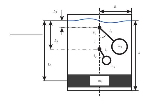
Fig. 1. Equivalent mechanical model approximating the liquid dynamics in a cylindrical vessel.
