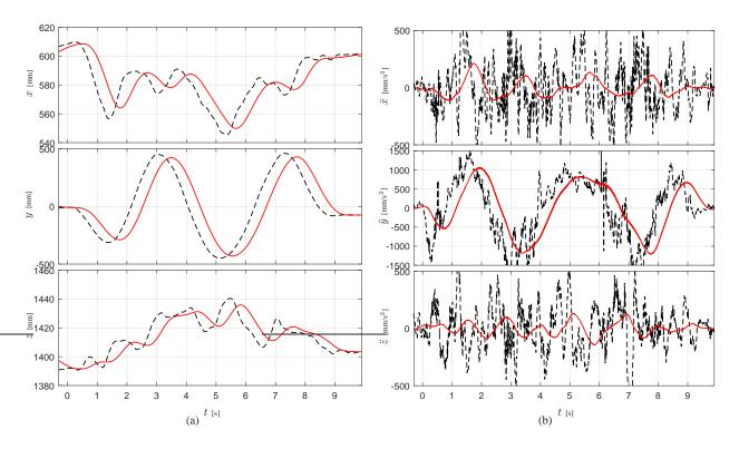
Fig. 11. Motion profiles corresponding to the geometric path of Fig. 10: positions (a) and accelerations (b). The black dashed lines are related to the original motion while the red solid lines represent the filtered trajectory.
