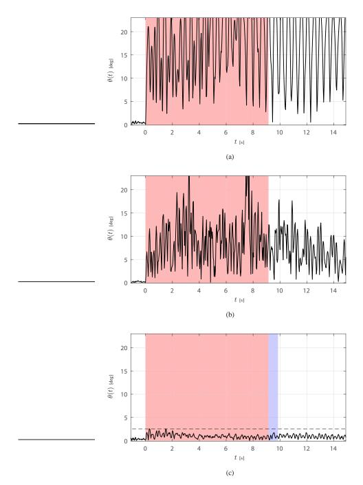
Fig. 12. Sloshing angle profiles measured when the liquid vessel is moved according to the trajectories of Fig. 11: unfiltered trajectory (a); unfiltered trajectory with orientation compensation (b); smoothed trajectory with orientation compensation (c). The red area indicates the motion time while the blue area highlights the time lag T introduced by the filter.
