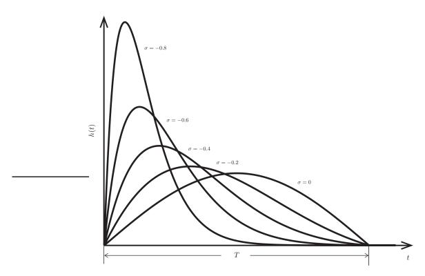
Fig. 3. Impulse response of the damped sinusoidal filter H(s) for different values of  $\sigma$ .
